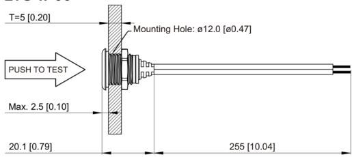
Dimension unit: mm [inch] Tolerance: ±1 [0.04]
